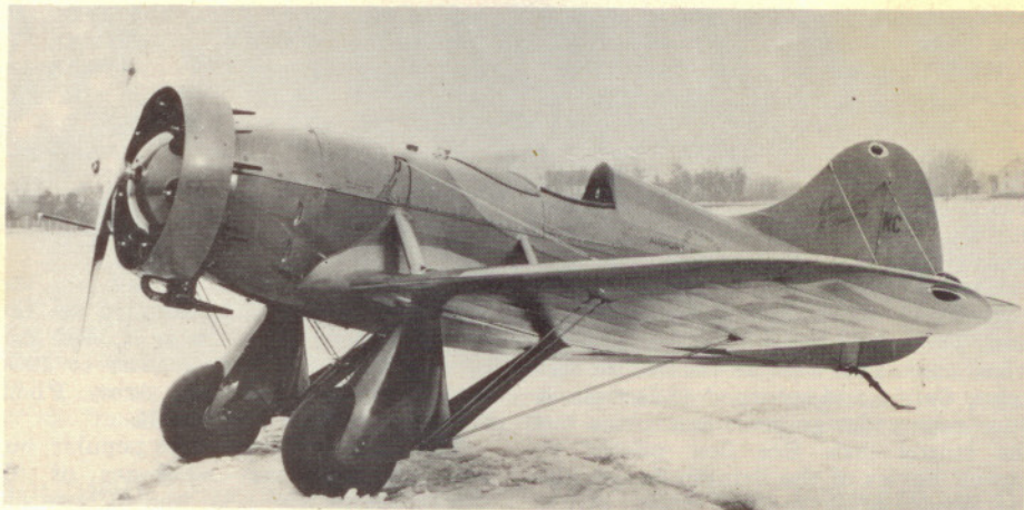
Improved Sportster was fitted with 110 h.p. Warner radial engine and designated Model E. More flying wires were used for added structural strength. Photos by the author
