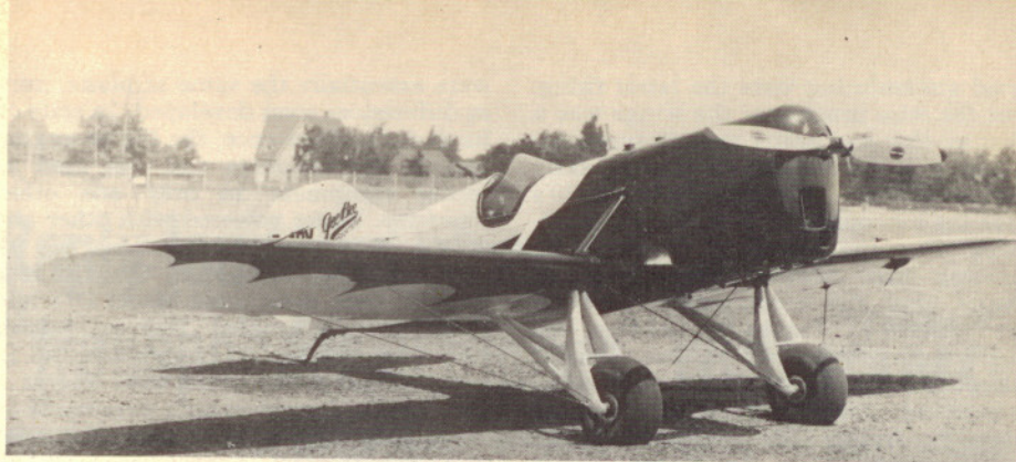
Original Gee Bee Sportster, designated Model X, had air-cooled Cirrus engine and rigid landing gear with Goodyear Airwheels. Wire wing bracing attached directly to axles.
